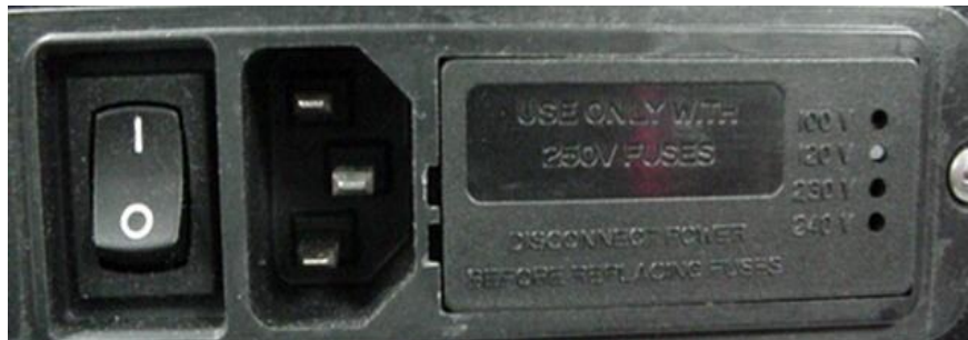
Figure 2. Power supply voltage selector, power cord connection, and on/off switch.
